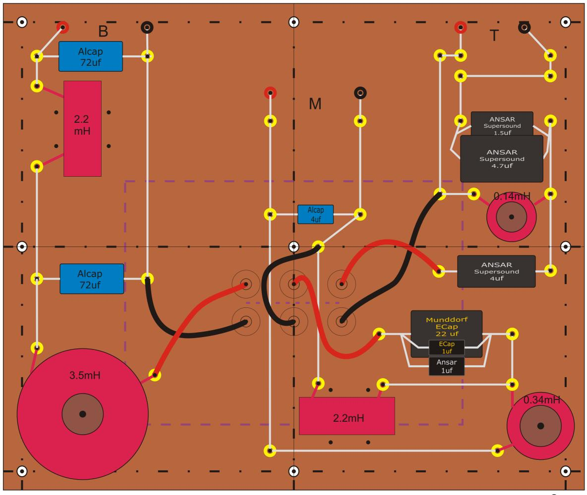
Stock coils are used but spacing is improved to avoid interaction, the board is 310 x 260 mm. This the largest that will fit through the driver aperture and it is located behind the ABR unit away from the large magnet on the Bass driver.
